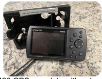
Garmin 496 GPS complete with antenna, Gizmo mounting bracket. Removed during upgrade.
