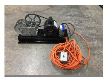
Hangar floor mount, GE 120v ac motor, 90ft steel winch cable, 75 ft control cable, \$125
