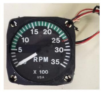
UMA 2-1/4 tach for use with Slick Magnetos (does not work with Bendix Magnetos).
