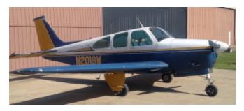
Total Time: 3,345 hrs.,. SPOH: 111 hrs. IO-470-K engine (225 HP), SMOH: 1,260 hrs KX-155 with Glideslope, MK-12D with GS Northstar GPS, KR-87 ADF, AT-150 & Encoder Standby Vacuum, Nov. '18 Annual \$54,450
